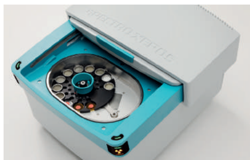
Illustration 2: Instrument measurement chamber with vacuum shutter
