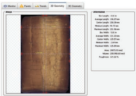
Overhead 2D measurements
